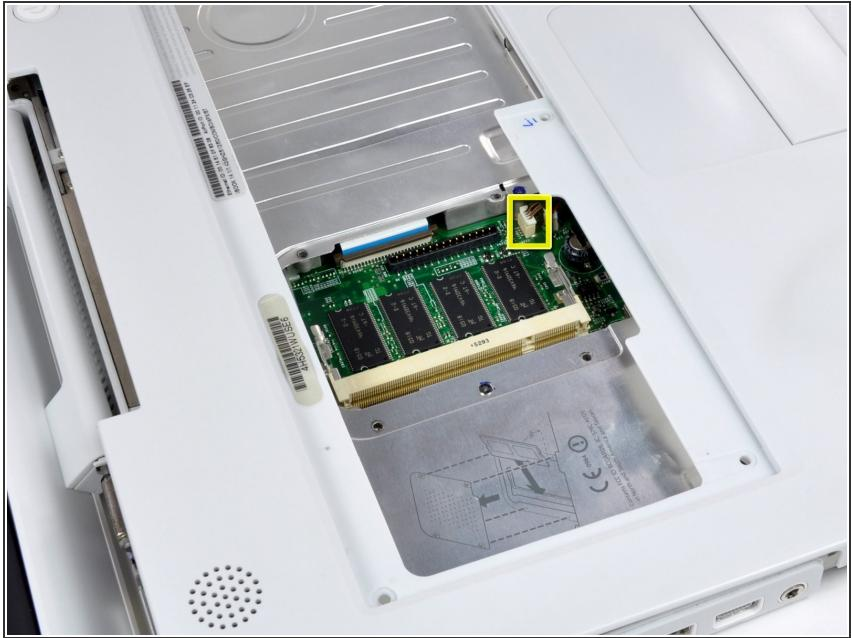
**i** Be especially careful while disconnecting the cables in the forthcoming steps. Never pull directly on the cables, but use a spudger to pry up the connector directly from its socket.
